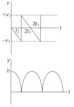
v = -gt and after the collision, v = gt (straight line).  $[\because v = u + gt]$  Collision is perfectly elastic, then ball reaches to same height again and again with same velocity.
